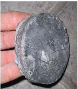
You will want to make a selection of "wafers" for different projects. Paint the wafer with paint to minimize lead chips from breaking off, and maintain the paint job. I use thick clear paint any good paint will work. Now get the Plexi-glass, cut out sections of the Plexi-glass that are about one-half inch larger all the way around, than the lead wafers.
