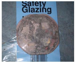
Make several sizes to work with different sized slabs, you can make different sized weights also. You will always want the Plexiglas to be larger than the slab you are trying to polish. Make sure corners are rounded, if they aren't they will hang up on the vibrating process. Now, take the Plexi-glass that is a bit larger than the wafer, center everything, and then epoxy the two together, with waterproof epoxy. Let dry very thoroughly.
